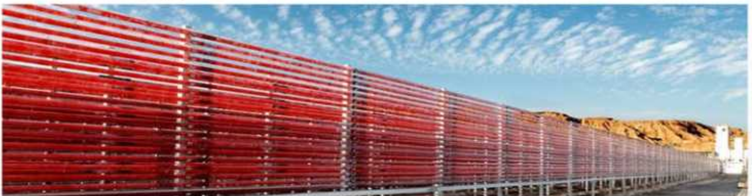
Fig. 2. Outdoor photobioreactor for the cultivation of Haematococcus pluvialis for the production of astaxanthin (source: https://www.scientistlive.com/content/high-quality-microalgae-products ) functions and properties of biopigments
